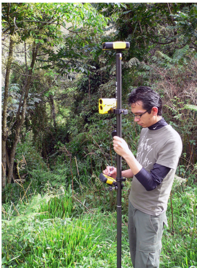
The technician Alberto Bravo carries out first measurements with the mobile DGPS unit. In the future we will provide an inventory of the most important installations, plots and sampling sites of the RU which already exist. Photo: Jörg Zeilinger.
